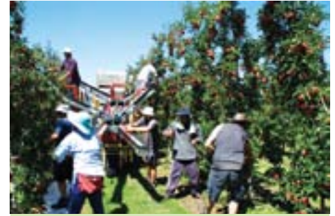
Apples are carefully placed onto the Zucal system elevators and gently make their way up to the fruit bin located at the rear of the platform.
