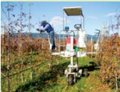
Tree training and pruning using the Trike battery powered platform. A recent addition was the solar panel on top of the Trike platform, which allows more working time in the orchard.
