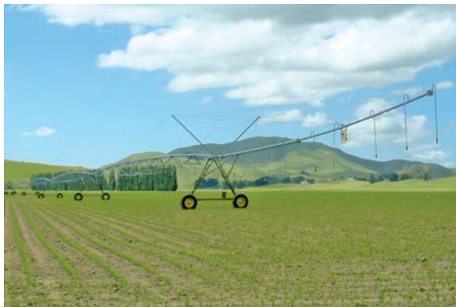
A 450 metre linear move irrigator is carefully managed to apply water only as required.
